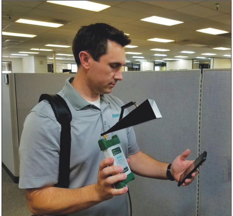
Figure 4. Millimeter-wave indoor coverage mapping solution.
