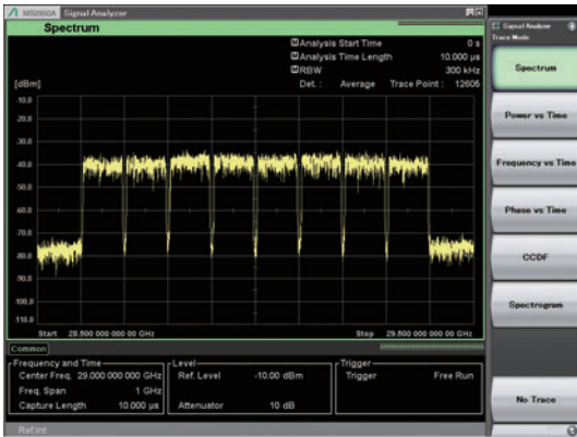
Spectrum of eight 100 MHz bandwidth carriers at 29 GHz center frequency
