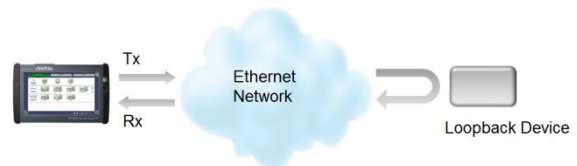
Fig. 5. Loopback Device Round-Trip Test
