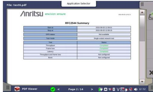
RFC 2544 Summary section with new table showing which tests completed
