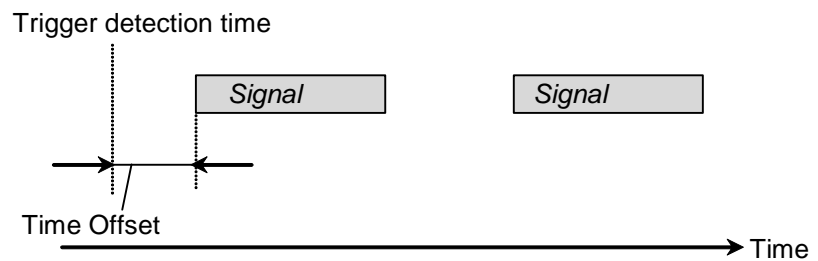
Figure 2.2.6-1 Definition of the timing error
