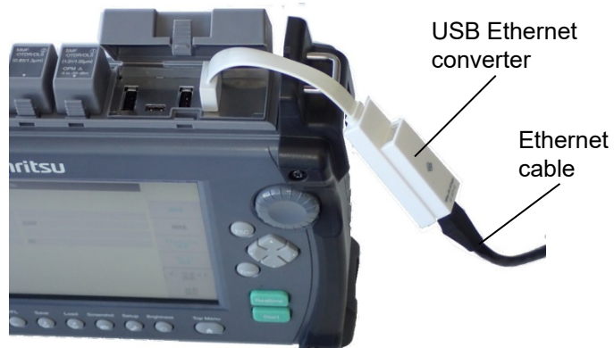
Figure 2.2.1-1 Ethernet Cable Connection
